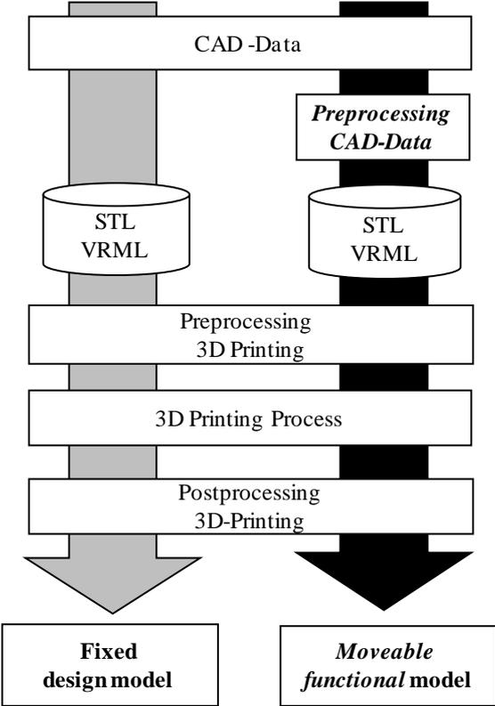
Figure 1. Design process for fixed models (left) and functional models (right)
