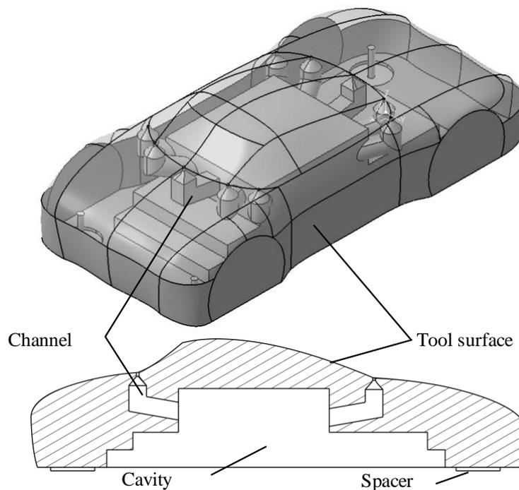
Figure 6. CAD model of a forming tool: 3D view and cross-section
