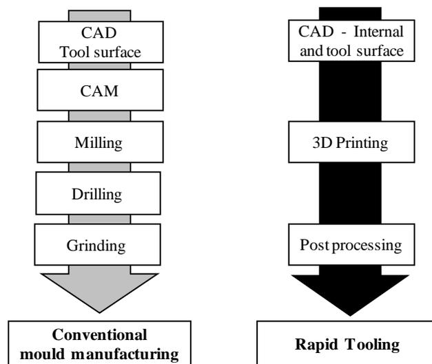
Figure 4. Conventional mould manufacturing and rapid tooling
