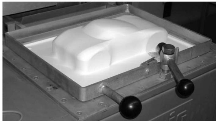
b. Thermoformed plastic sheet
